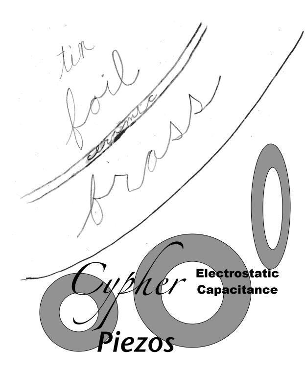
Piezos are sandwiches of brass and ceramic, glued together with epoxy and then sprayed with a thin tin foil on top. When you play your bars really hard, this very thin ceramic can break and the piezo can become leaky to ground, resulting in a cypher, or ghost tone.
