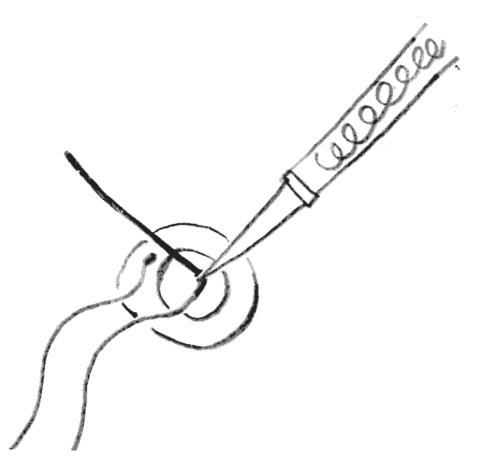
Note- you can add extra piezos to supercharge a barre! Just glue more on and repeat this process with little jumper wires to make a parallel circuit with them.
